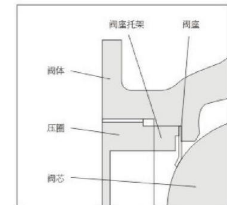
图2 铜片式金属硬密封结构局部图 Figure 2 Steel sheet type metal hard seal structural diagram
